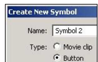
To create a Button, right-click on the Library, and choose New Symbol. Give the Symbol a name, and set the Type to Button. The stage will now be replaced with the Symbol Editor pane. Again, use the tools to create a button. While the Timeline for a button has Layers, it also has four main frames – Up, Over, Down and Hit.
